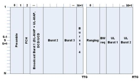
Figure 6: OFDM Frame Structure: Example From Standard
