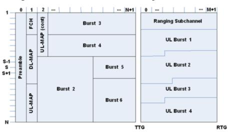
Figure 7: OFDMA Frame Structure: Example From Standard
