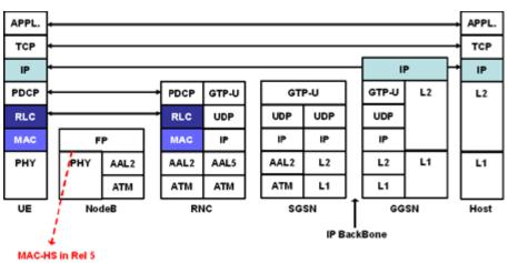
Figure 3: UMTS Protocol Architecture (User Plane)
