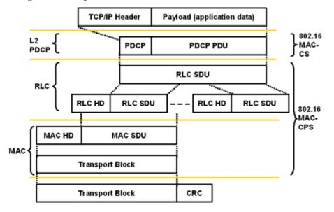
Figure 4: Comparison of UMTS & 802.16 Protocol Architectures
